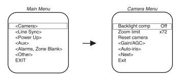
NOTE: If backlight compensation is ON and the IR cut filter switches OUT (black and white mode) in normal lighting conditions, adjust the Auto IR Level to a darker setting. Refer to the Auto IR Level section. There are two backlight compensation modes:
